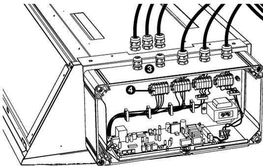
3. Lead the control cable(s) into the box through the free cable gland(s) ❸.
