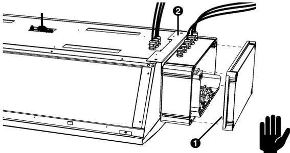
1. Remove the cover ❶ from the box on the side of the unit.
