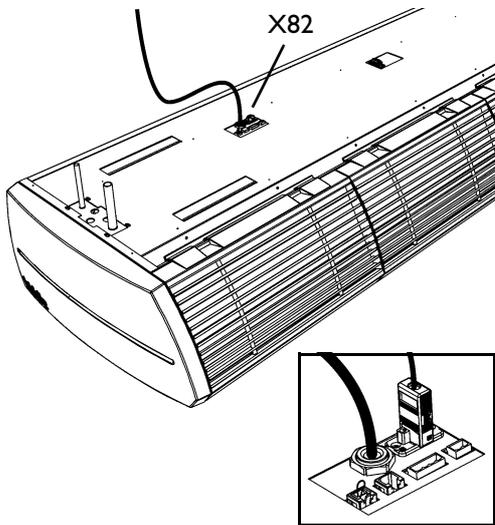
1. Attach the outside air temperature sensor to the outside of the building.
