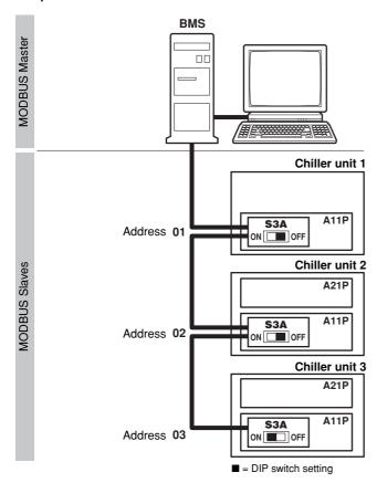
In this example, the last in line DIP switch on the address cards of chiller units 1 and 2 are to be set to OFF. Because chiller unit 3 is the last unit in line, the last in line DIP switch on the address card must be set to ON.
