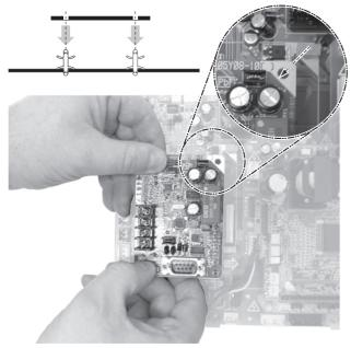
Make sure that the address card is firmly fixed. The heads of the spacers must be properly pushed through the mounting holes located at the 4 corners of the address card.
