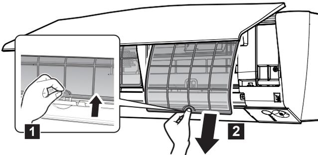
**Class 40:** The titanium apatite deodorising filter and the silver particle filter (Ag-ion filter) **MUST** be removed before cleaning the air filter.
