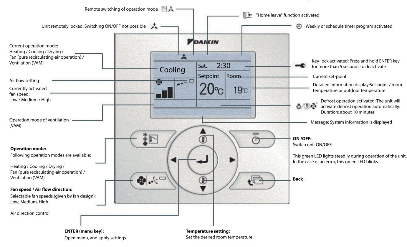
Press and hold for more than 5 seconds to activate key-lock. Press and hold again for more than 5 seconds to deactivate key-lock.
