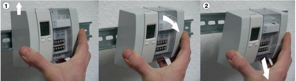
Fig. 25: Removing the base module from the top-hat rail
