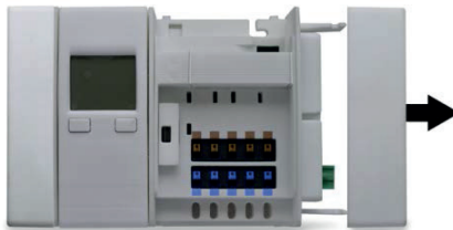
Fig. 10: Pulling off the closing cap.
