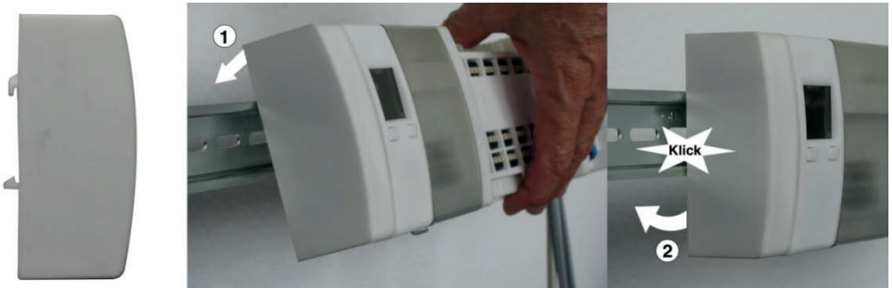
Fig. 24: Mounting on the top-hat rail
