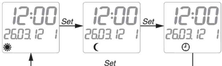
Fig. 33: Navigation structure of mode ("Set") day, night and clock
