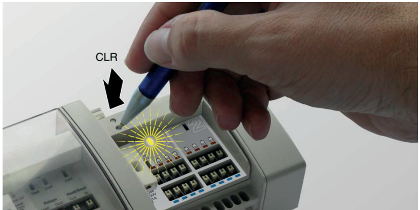
Fig. 28: Clearing the controller module
