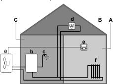
Gas boiler (\*HY2KOMB28+32AA) + domestic hot water tank
